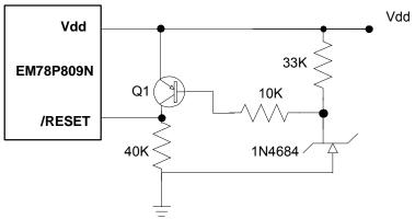
Fig. 36. Residue Voltage Protection Circuit 1
